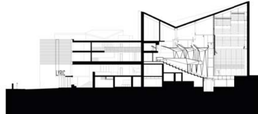
SECTION CUT THROUGH MAIN AUDITORIUM
